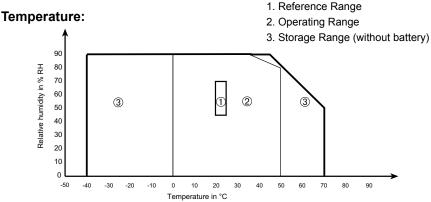
**Operating Temperature:** 32 to 122°F (0 to 50°C); 90% RH **Storage Temperature:** -40 to 158°F (-40 to 70°C); 90% RH
